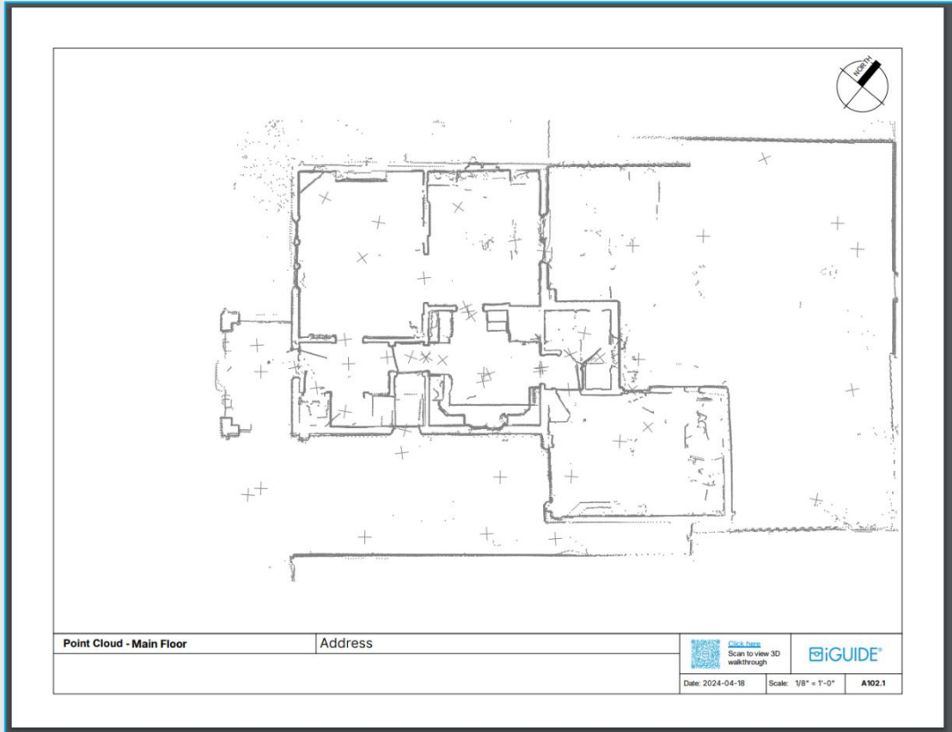
Figure # 36 - Point Cloud - Main Floor
